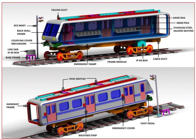
The indicative picture as shown above has been provided to give a clear understanding about our products, its uses and places of installation. The picture depicts the diagram of a Metro Rail Coach and also represents the uses and places of installation of our manufactured products in a Coach (Interior and Exterior).
